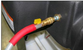
Attach the machine's **BLACK** vacuum hose with open end adapter to the vehicle's overflow nipple at the radiator cap and open ball valve.
