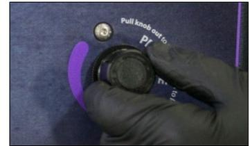
Slowly open the valve on the **YELLOW** pressure hose. Fill to desired level and close valve.
